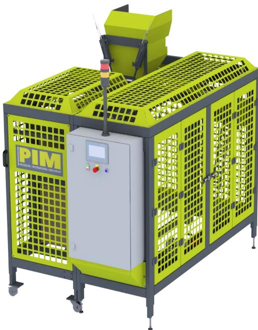
The Automatic Bag Placer is a compact and cost efficient solution to fully automate the process of packaging products in single bags. The ABP is designed to be integrated with a packaging machine taking over the manual operations, greatly increasing the efficiency of packing single bags while still keeping the possibilities to quickly switch between packaging type or size.
