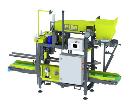
The Semi-Automatic Sewing machine is the solution for bag filling followed by an automatic closing of the opening using high quality sewing equipment. Designed specifically for loose single bags and manually adjustable for high variety of bag dimensions. The SAS is easy to operate and can be easily integrated with your weighing and packaging lines.
