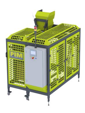
The Automatic Bag Placer is a compact and cost efficient solution to fully automate the process of packaging products in single bags. The ABP is designed to be integrated with a packaging machine taking over the manual operations, greatly increasing the efficiency of packing single bags while still keeping the possibilities to quickly switch between packaging type or size.
